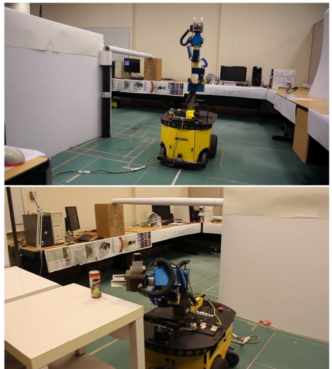
Fig. 8. Real environment for pick-and-place task. The mobile manipulator start configuration and object (bottle) are shown in the top figure while the bottom figure shows the table on the other side of the door where object should be placed.
