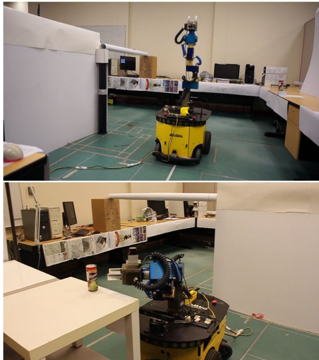
Fig. 13. Real environment for pick-and-place task. The mobile manipulator start configuration and object (bottle) are shown in the top figure while the bottom figure shows the table on the other side of the door where object should be placed.
